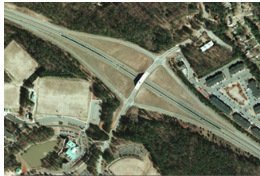
Figure 7: Full Diamond Interchange
